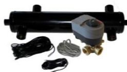
Hot Water Priority kit ¾" (SKU:300040, 300041) Produces hot water only when it is needed. Closes hot water tank, when the house is heated. Kits available with either 2 or 3 way motorized valve.
